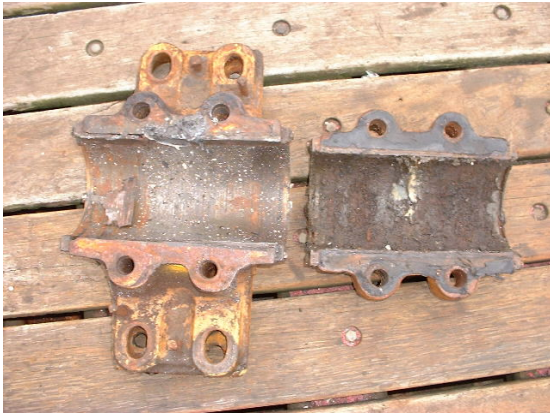
Failed Lead Babbitt Shaft Bearing
